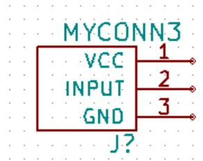
28. It is time to place the power and ground symbols. Click on the *Place power port* button
