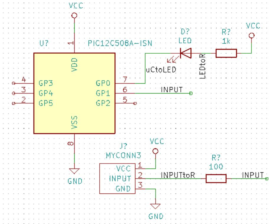
40. Let's now deal with unconnected wires. Any pin or wire that is not connected will generate a warning when checked by KiCad. To avoid these warnings you can either instruct the program that the unconnected wires are deliberate or manually flag each unconnected wire or pin as unconnected.
