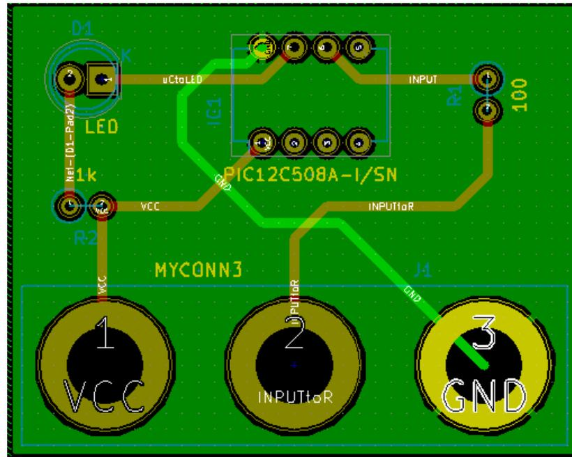
25. Run the design rules checker by clicking on the *Perform design rules check* icon
