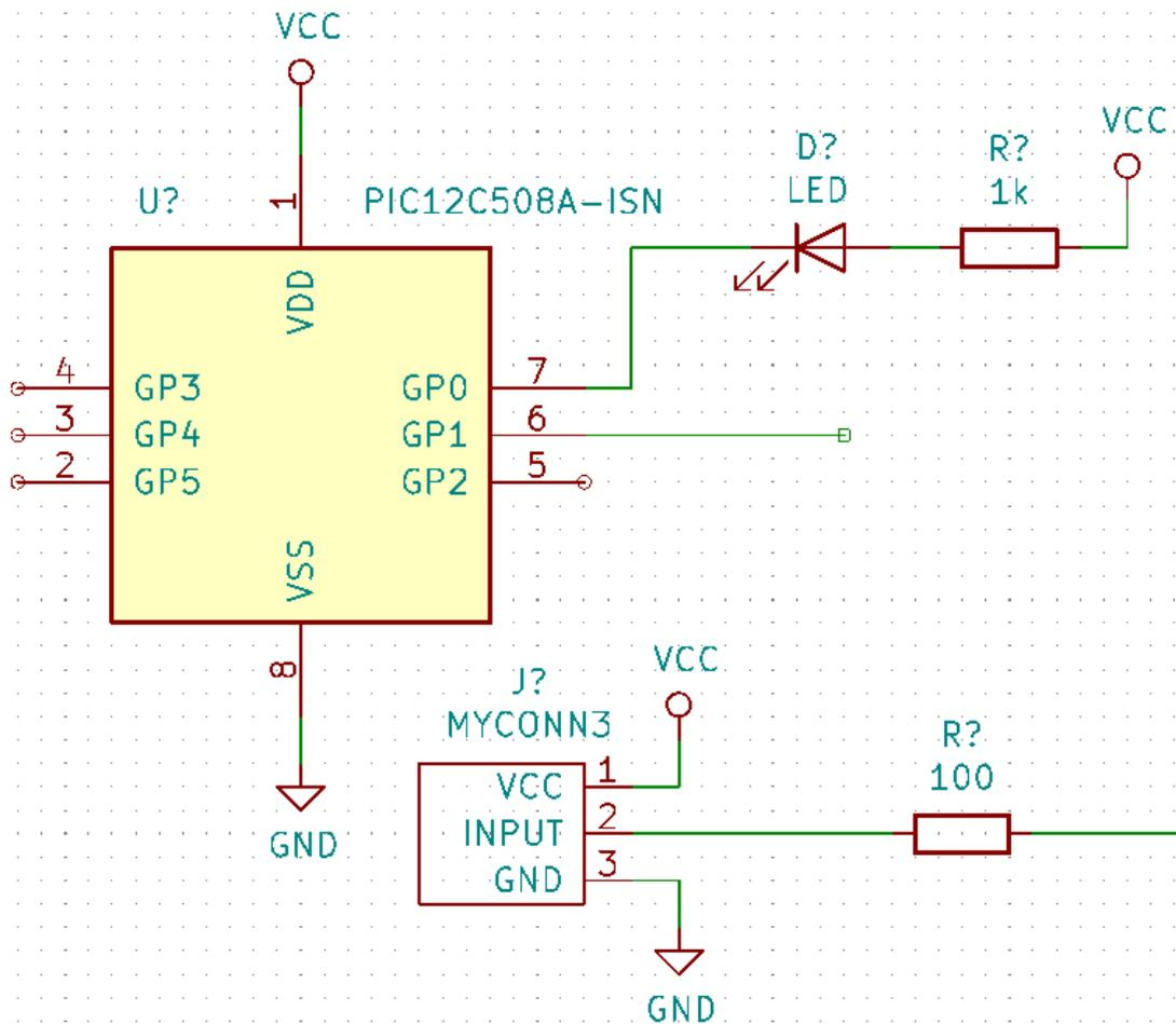
34. We will now consider an alternative way of making a connection using labels. Pick a net labelling tool by clicking on the *Place net label* icon
