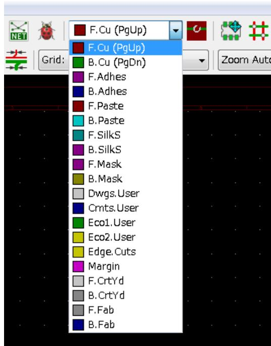
14. If you decide, for instance, to do a 4 layer PCB instead, go to **Setup** → **Layers Setup** and change *Copper Layers* to 4. In the *Layers* table you can name layers and decide what they can be used for. Notice that there are very useful presets that can be selected via the *Preset Layer Groupings* menu.
