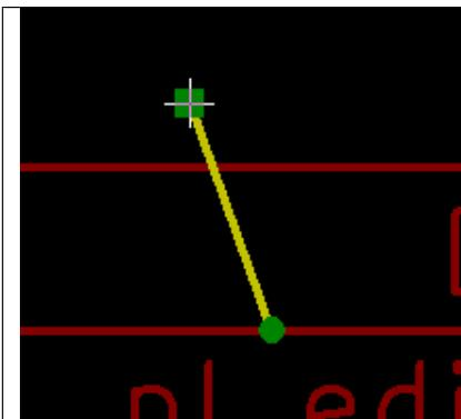
Once selected, the item, or one of its end points, can be moved by moving the mouse and placed (right clicking on the mouse).
