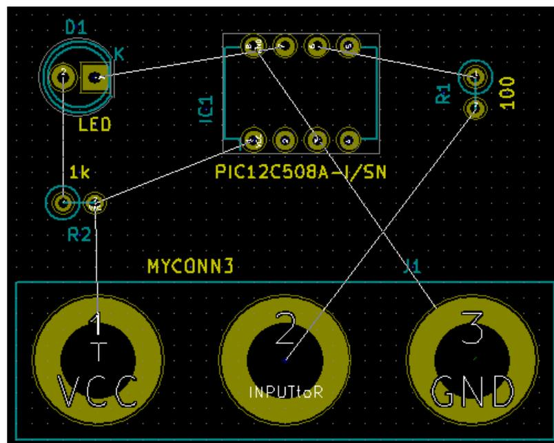
10. Note how one pin of the 100 ohm resistor is connected to pin 6 of the PIC component. This is the result of the labelling method used to connect pins. Labels are often preferred to actual wires because they make the schematic much less messy.
