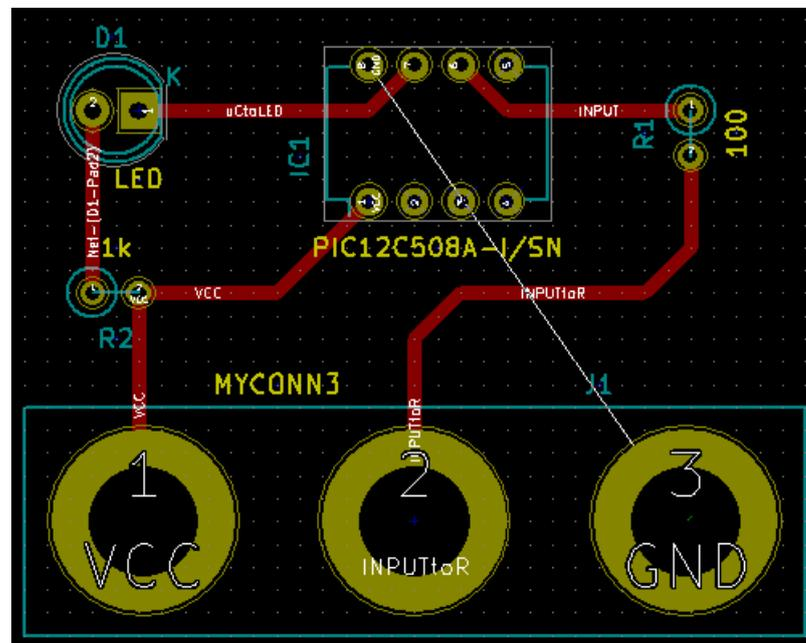
20. Let's now run a track on the other copper side of the PCB. Select *B.Cu* in the drop-down menu on the top toolbar. Click on the *Route tracks* icon
