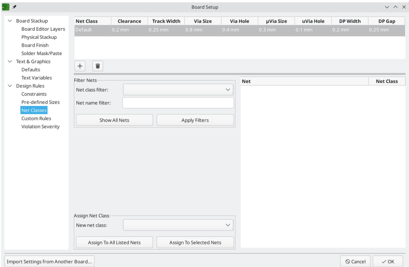
Track width and spacing can be managed manually by the designer during layout, but net classes are recommended because they provide an automatic way to manage and check design rules.
